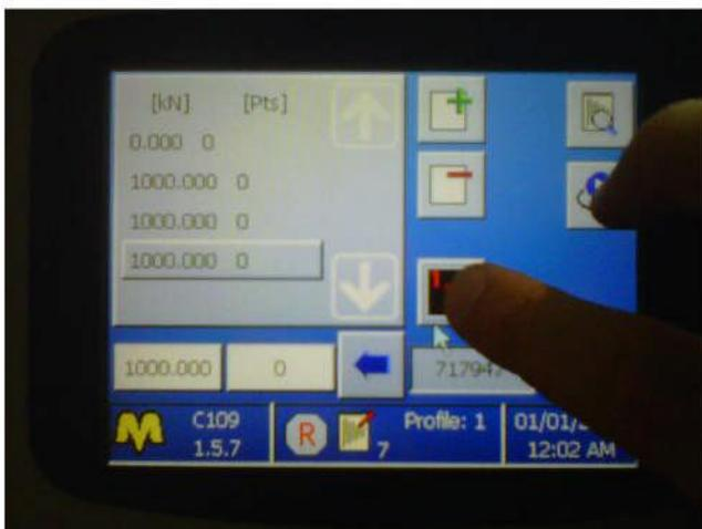
Once the force steps have been defined, press the blue vertical arrow on the right of the screen to access to the following view (picture above).
