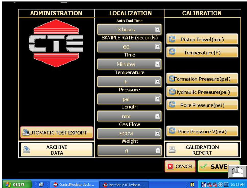
This menu option allows the user to calibrate the pressure transducers, or other devices, if necessary. The procedure uses a dead weight tester or compressed gas and a certified pressure transducer to calibrate the transducer. Follow the steps below to calibrate the hydraulic pressure transducer. The steps are similar for the other devices.
